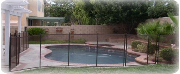
**Straight or Curved?** A straight pool fence is easier and cheaper to install than one that curves in and out.
